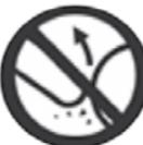
Contact of the guide bar tip with any object should be avoided.
