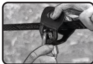
Attach Carabiner to Roller
