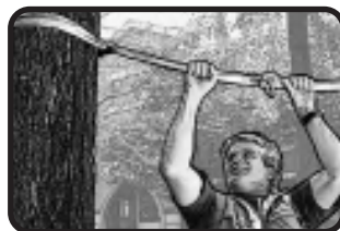
Coil Line under Ratchet
