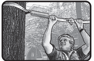
Mandatory Load Test Pull on Line to test it on both ends.
