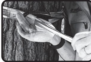
Coil Line under Ratchet
